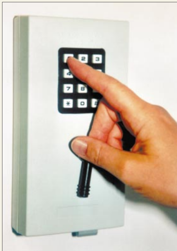
MST Chrontec keypad module with integrated TIRIS reader.
